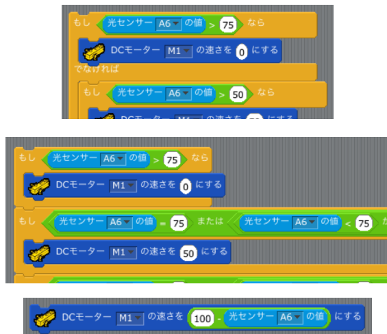
図 16 明るさに応じて LED の明るさを変えるプログラム Fig.16 Program code to change LED brightness according to the surrounding brightness
